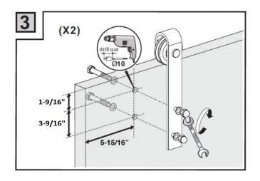
Drill out holes in the door using a 10mm routing drill bit as pictured.
