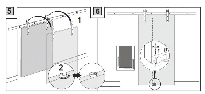
Attach the doors to the rails making sure that the anti-jump disks are engaged to avoid a serious accident.
