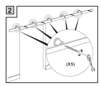
Attach the rail to the wall brackets using a wrench to fasten the bolts as shown.
